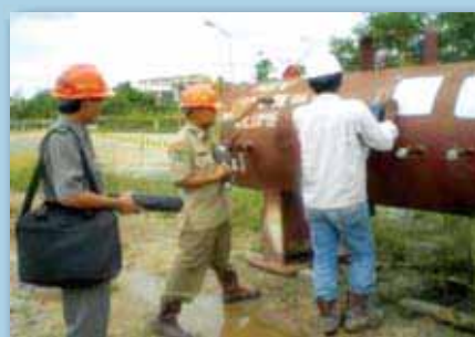
Air Pressure Tank Inspection by Depnaker
